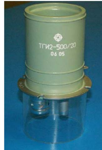
Note: the thyratrons operate at pulse repetition rate to 50000 pulse/s on condition of decrease of pulse and average power.
